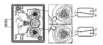
Make the electrical connections in compliance with the rules in force, paying attention that, during operation, the cables do not interfere with the cams and the gears.
